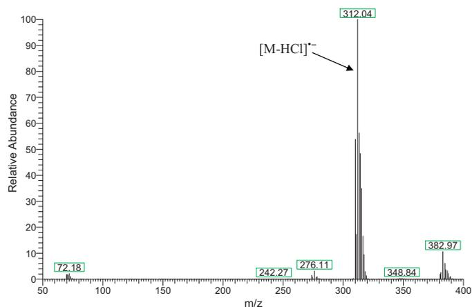
**Fig. 1.** ECNI mass spectrum of 1,2,5,6,9,10-hexachlorodecane at ion source temperature of 150 °C.
