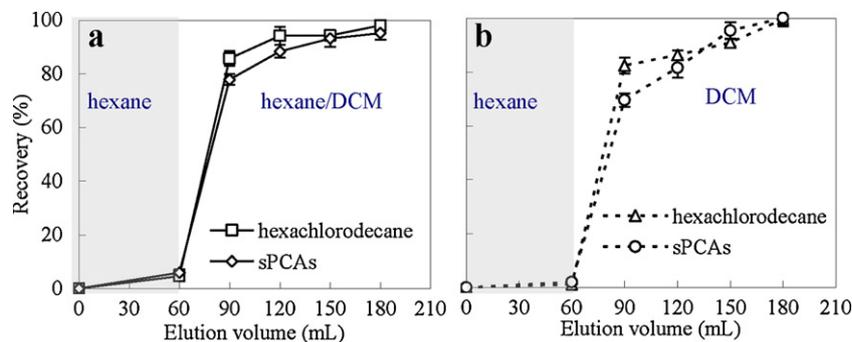
**Fig. 2.** The elution curves of 1,2,5,6,9,10-hexachlorodecane and sPCAs with 55.5% chlorine content on (a) neutral alumina column (first eluted by 60 mL hexane, then 120 mL 1:1 hexane/DCM) and (b) basic alumina column (first eluted by 60 mL hexane, then 120 mL DCM).
