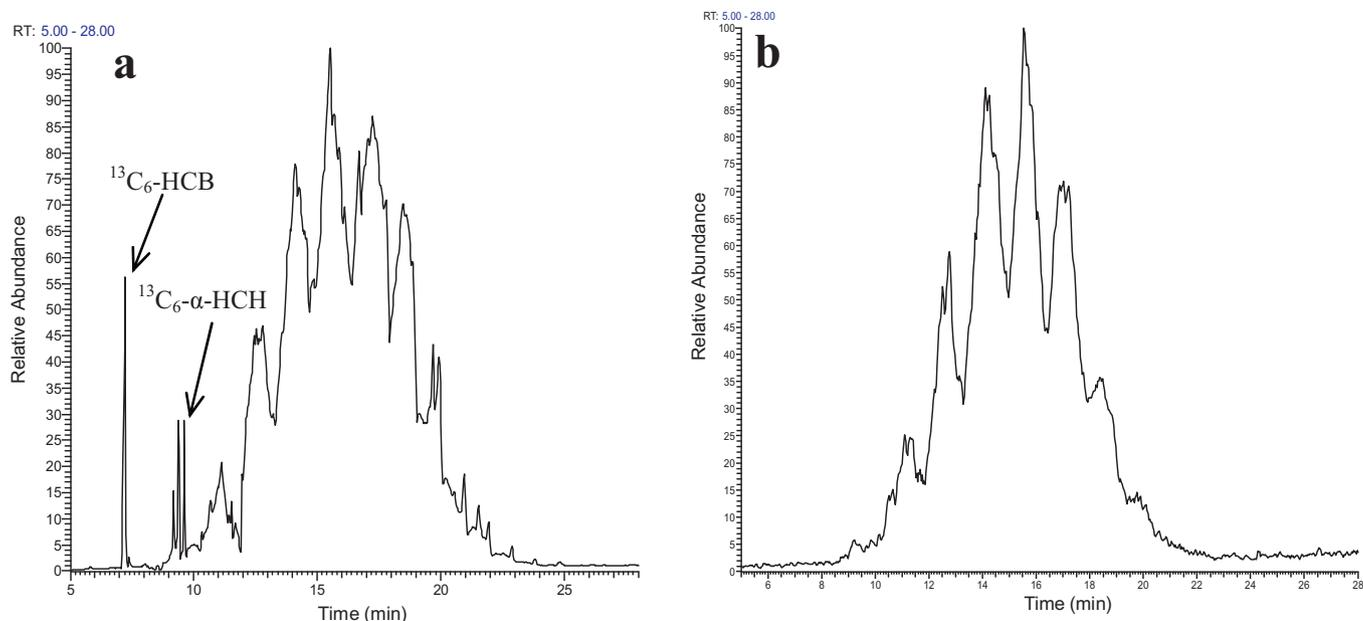
Fig. 3. Chromatograms of sPCAs (a) in a sediment sample pretreated by the optimized cleanup method and (b) in an sPCAs stock solution with 55.5% chlorine content.
