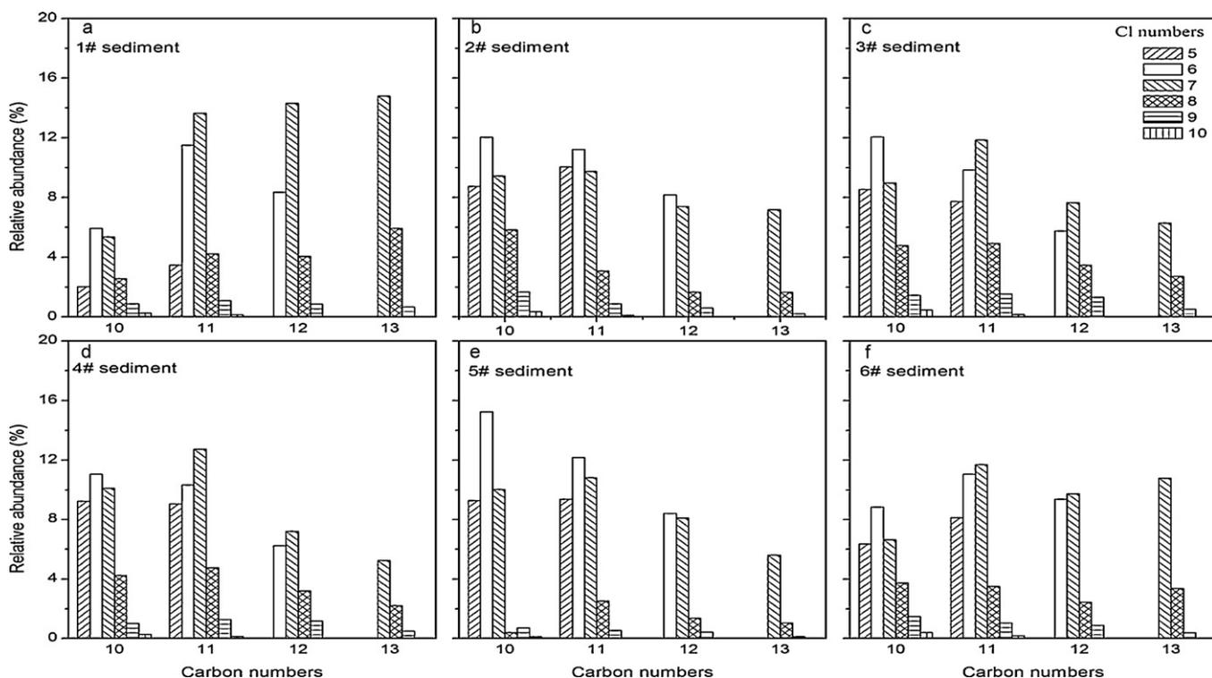
Fig. 4. Homologue pattern ( $\text{C}_{10}$ – $\text{C}_{13}$ ) of sPCAs in sediment samples from the mouth of the Daliao River determined by HRGC/ECNI-LRMS.
